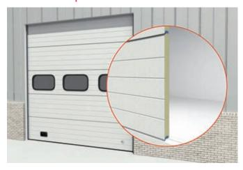
The Loading Systems traditional industrial panel is provided with an in-built thermal break. The tongue and groove design ensures an almost seamless seal between the panels preventing air and/or water from penetrating through the seals, ensuring the best possible insulation properties.
