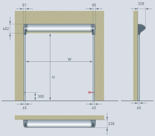
All indicated dimensions are based on exact width and height dimensions only. The space necessary for mounting and maintenance has to be provided.
